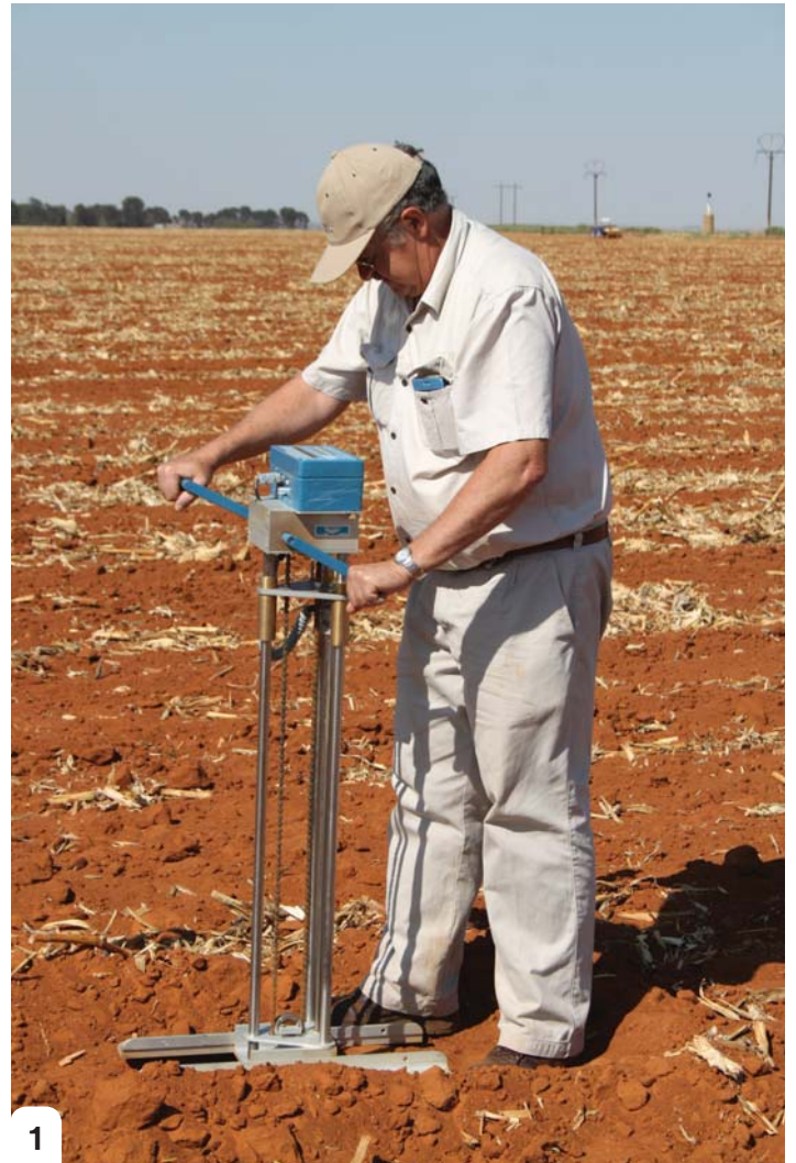
1 A soil scientist performing soil compaction tests by means of a penetrometer.
