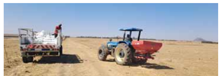
Ranko Tsotetsi from Kestell was busy spreading lime when mentor Johan Roux, paid him a visit. Johan and Ranko recalibrated the spreader again after Ranko discovered that the quantity that was spread, was more than what was calibrated. They found that the driver was driving too slowly, so the RPM was adjusted to 1 500, which solved the problem. ■
